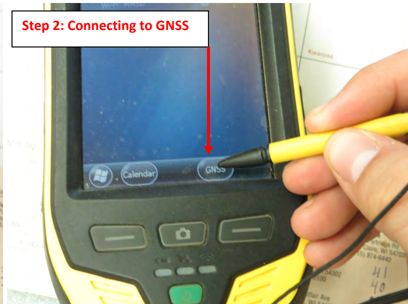
Step 4: Using the pen click on GNSS and wait for satellites to be found.
