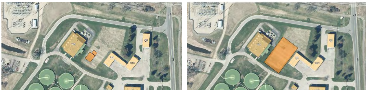
Figure 5. Possible Location for TP Treatment at NSW WTP (Top), Clearas footprint (Left), BluePro footprint (Right)
