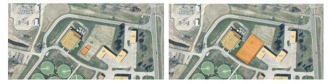
Figure 5. Possible Location for TP Treatment at NSWWTP (Top), Clearas footprint (Left), BluePro footprint (Right)
