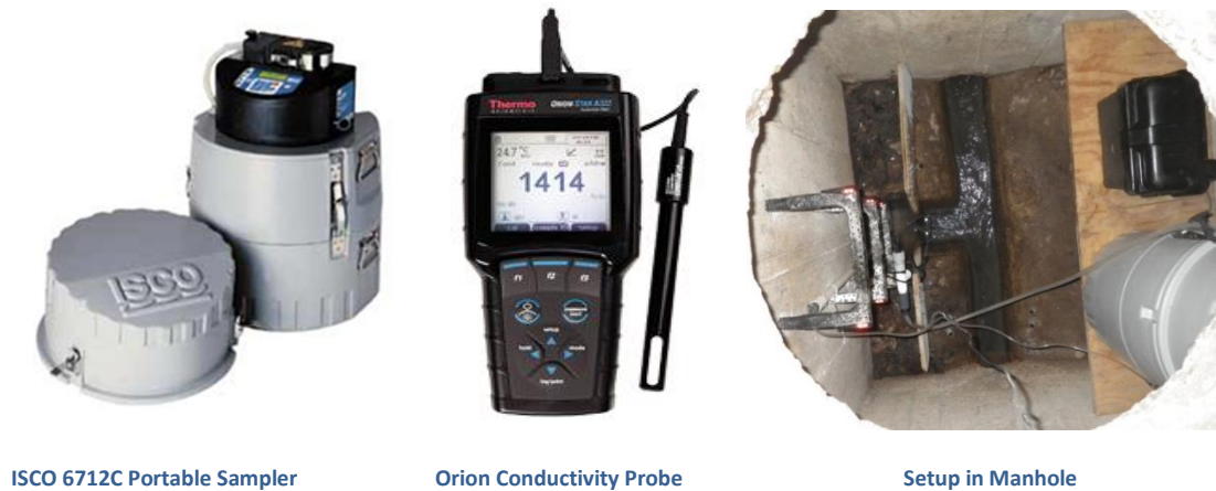
Figure 4 Manhole Monitoring Equipment and Setup
