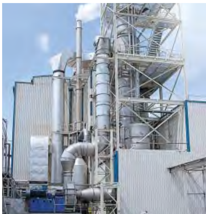
1-effect falling film evaporation plant heated by mechanical vapour recompression for wheat starch effluent. Evaporation rate: 17,000 kg/hr
