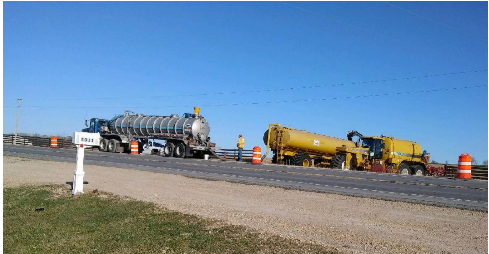
Setup along Hwy 19 (left to right) Metrogro tanker, nurse tank, Terragator
