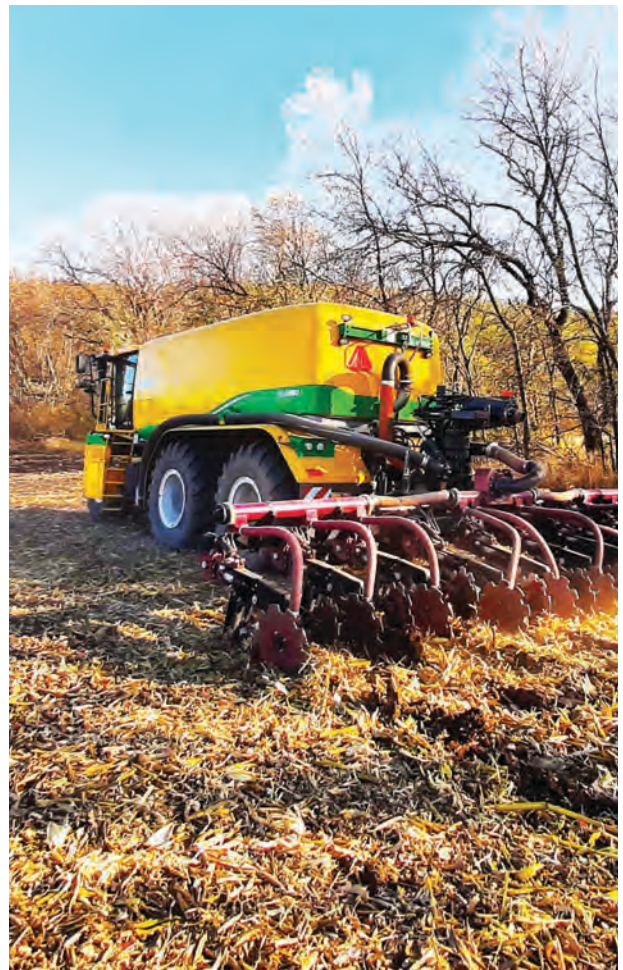
The District's new Metrogro applicator use low-disturbance injection equipment.
