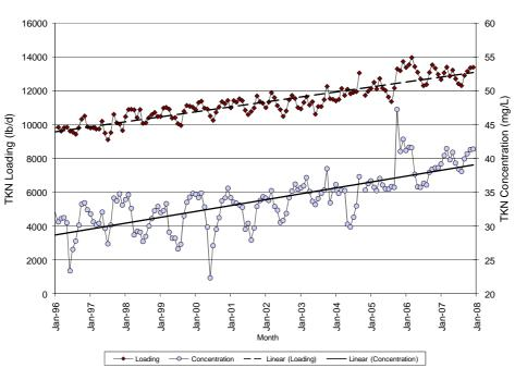
Figure 2-4. Raw Wastewater TKN Loadings & Concentrations - Monthly Average (1996-2007)
