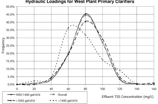
Figure 4-2. Effluent TSS Concentration Frequency Distribution at Various Hydraulic Loadings for West Plant Primary Clarifiers
