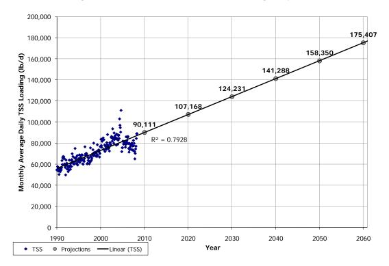
Figure 3-2. Raw Wastewater TSS Loading Projection
