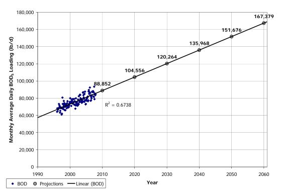
Figure 3-1. Raw Wastewater BOD<sub>5</sub> Loading Projection
