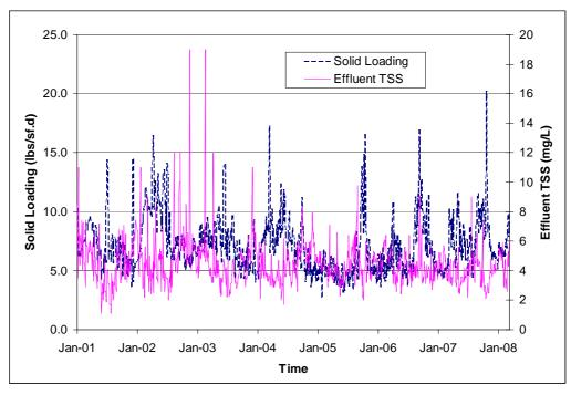
Figure 4-4. Plant 2 Secondary Clarifier Performance (2001-2008)
