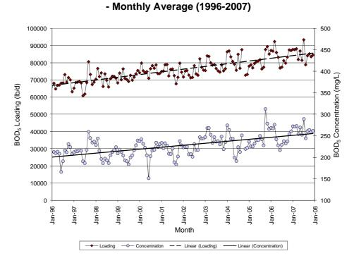
Figure 2-2. Raw Wastewater BOD<sub>5</sub> Loadings & Concentrations
