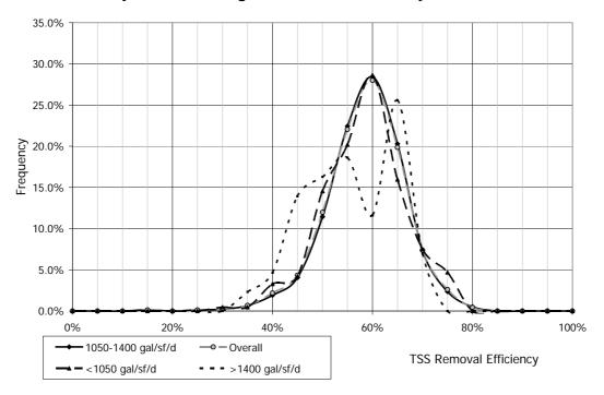
Figure 4-1. TSS Removal Efficiency Frequency Distribution at Various Hydraulic Loadings for West Plant Primary Clarifiers
