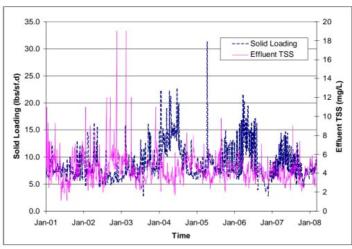
Figure 4-3. Plant 1 Secondary Clarifier Performance (2001-2008)
