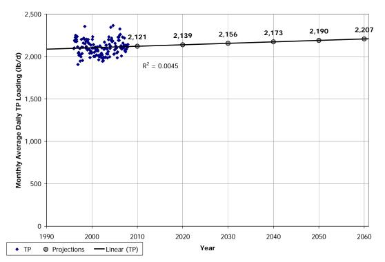
Figure 3-4. Raw Wastewater TP Loading Projection
