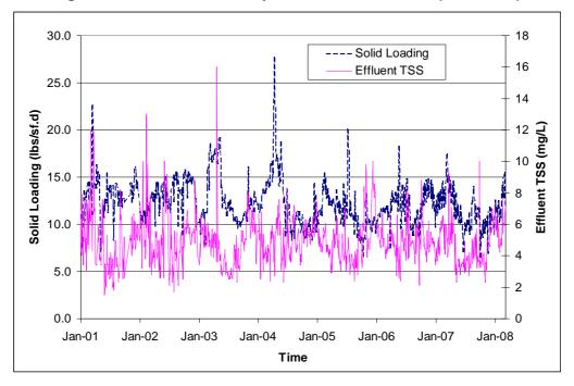
Figure 4-5. Plant 3 Secondary Clarifier Performance (2001-2008)
