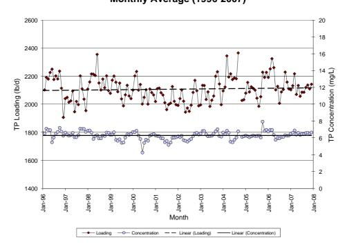
Figure 2-6. Raw Wastewater TP Loadings & Concentrations - Monthly Average (1996-2007)
