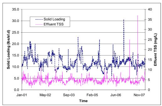
Figure 4-6. Plant 4 Secondary Clarifier Performance (2001-2008)
