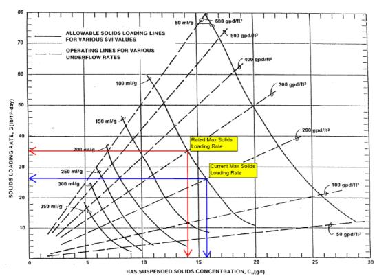
Figure 4-7. Secondary Clarifier Solids Loading Capacity Estimation
