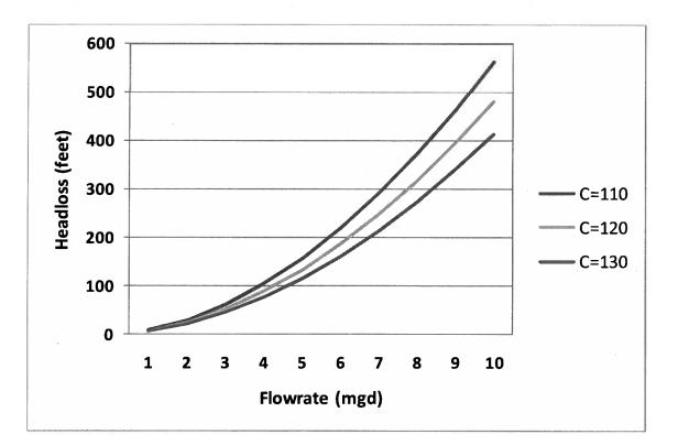
The headloss at different flow rates and Hazen-Williams roughness factors are shown in Figure C-1 and Table C-2.
