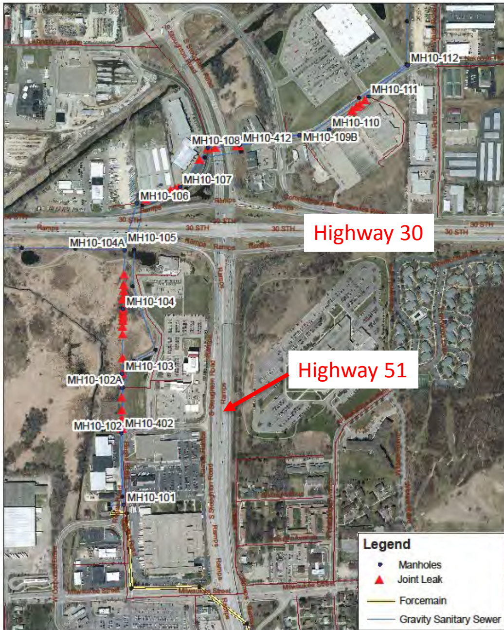
MH10-101 to MH10-112 Joint Leaks
