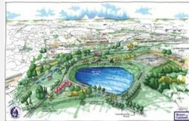
One promising option being evaluated on Starkweather Creek involves efforts by the city and its consultants to bind and settle phosphorus to the bottom of a stormwater pond so the phosphorus does not reach Lake Monona. The project is testing a variety of coagulants and dosing rates. While these practices are new to our region, the work leverages experts and research findings from throughout the country.
